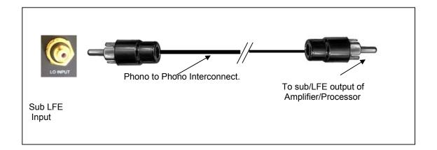
Connect as shown above using a phono to phono interconnect. Plug one end into the sub/LFE output on the amplifier/processor and the other end into the LFE LEVEL input on the sub-bass system.
